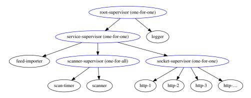
Supervision tree of a real-life application (processes can be spread on remote nodes)
