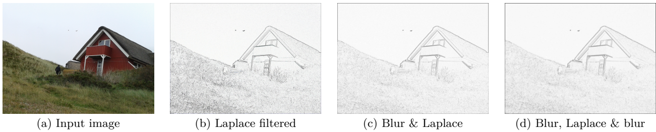
Figure 1: Input image and results from using edge detection via a Laplace operator.
